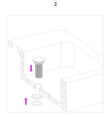
2.Put the main body down from the basin, and install the gasket from the basin to the main body
