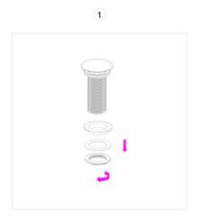
1.Disassemble the gasket and nut of the drainer according to the figure.
