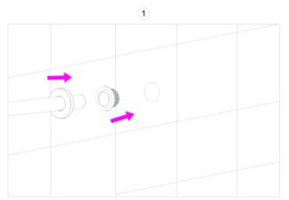
1.Put the plastic plug into the wall, then put the straight pipe into the plastic plug, push the rosette to the wall.
