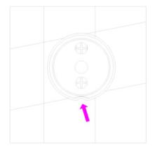
2. When installing the fixed seat, pay attention to the installation direction. The two screw holes should be parallel with the ground.
