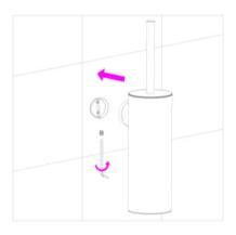
3.Install the main body with the fixed seat, then lock the screws with the hexagon key.
