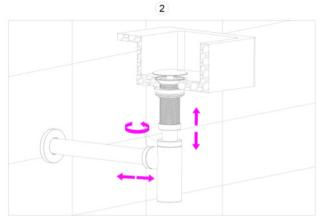
2.Both fixed cover for sifon,Adjust the length according to the distance of the table, then connect the screw teeth of the table, and then fix the two fixed covers tightly after installation.
