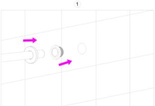
1.Put the plastic plug into the wall, then put the straight pipe into the plastic plug, push the rosette to the wall.
