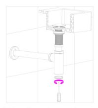
If clean the push up waste, open the bottom cover of the waste with a screwdriver.
