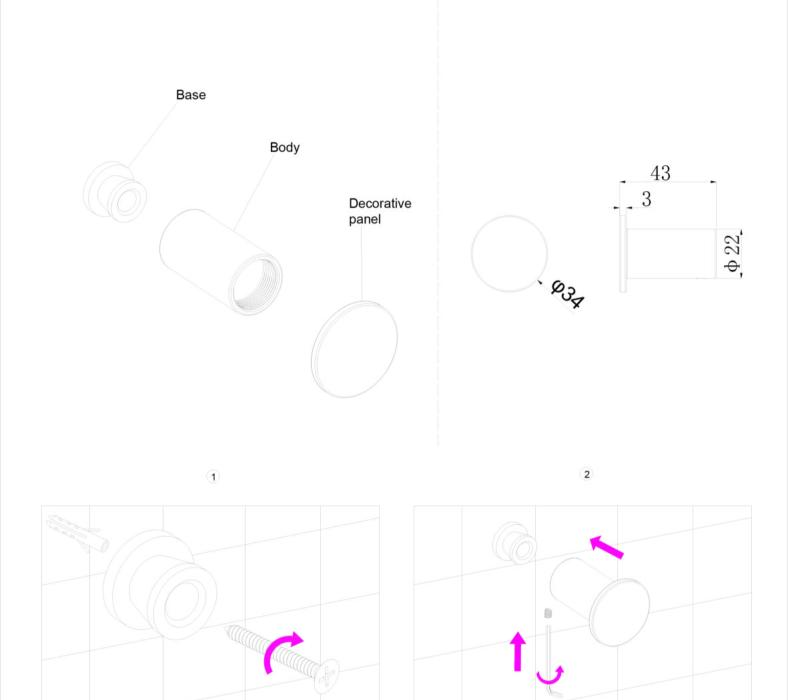
1.Fix the base to the wall with a self-tapping screw.
