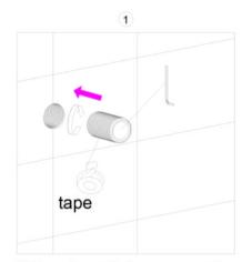
1.Wrap the white tape around the connecting rod screw, then fix the connecting rod to the wall with a hexagon spoon.
