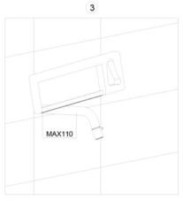
3. The spout length can be resected according to the need, and the maximum resected length should not exceed 110mm.
