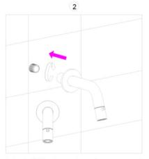
2.Install the faucet on the connecting rod and then push the cover plate against the wall until it is close to the wall.
