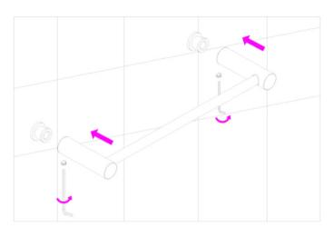
2.Install the hanger rod at the base of the wall and then lock the screws with the hexagon key.
