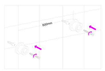
1.Mark the size with a pen on the wall and fix the base on the wall with a tapping screw.
