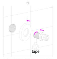
1.Wrap the white tape around the connecting rod screw, and then use the allen key to fix the connecting rod to the wall. Pay attention to install the rosette first.
