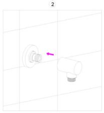
2. Install the main body to the installed connector.
