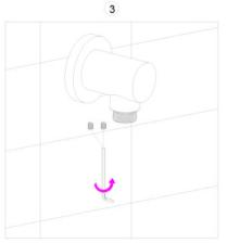
3.Fix the main body with screws at the bottom.
