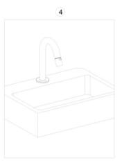
4.After installation, swing the outlet pipe from side to side and test whether each connection is leaking or not.
