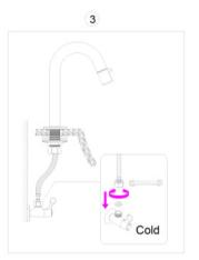
3.Install the two side connector of the hose on the faucet and valve.
