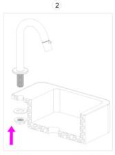
2. Fixed the spout into the mounting hole and install the gasket and lock nut at the bottom.
