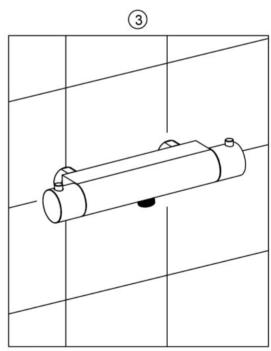
3.Install all parts according to the picture. After installation, Testing whether each connection is leaking or not
