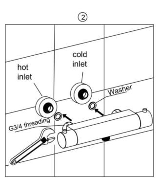
2.Put the washer into the nut and tighten the nut with a wrench.
