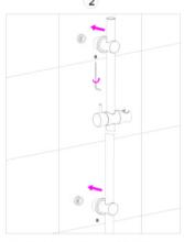
2.Align the two lifting fixing seats with the base and fix them with the hexagon key.
