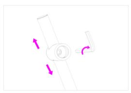
Tip: After loosening the screws from behind the base, adjust the base position up and down.
