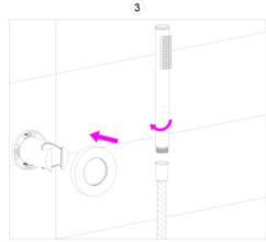
3.Install the cover plate into the socket, install the handshower and hose.
