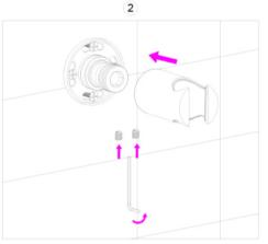
2.Install the socket into the connecting rod and secure it with the hex key twist screw.
