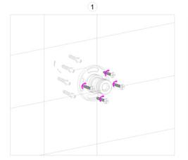
1.Fix the base to the wall with a self-tapping screw.
