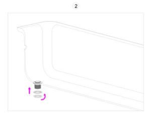
2.Use the screw of drainer to connect the parts according to the figure.
