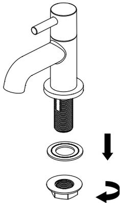
Unscrew the mounting nut and rubber washer from the tap.
